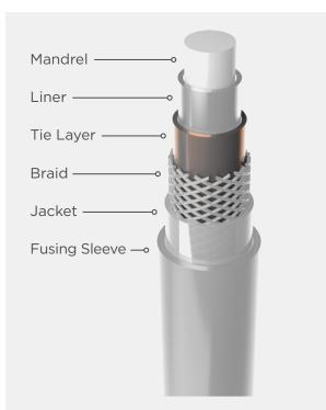
Tie Layer creates a melt-bondable surface that improves adhesion to both the liner and catheter jacket during the reflow process.
